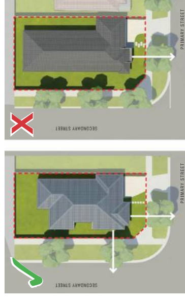
FIGURE 2 - CORNER LOT FACADE DESIGN
