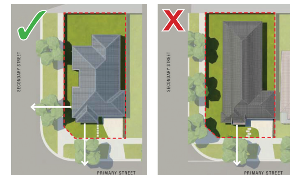
FIGURE 2 - CORNER LOT FACADE DESIGN
